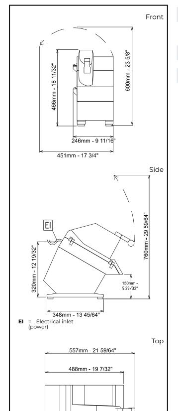
Electric 220-240 V/1N ph/50 Hz Supply voltage: Electrical power, max: 0.37 kW **Total Watts:** 0.37 kW Capacity: Performance (up to): 400 kg/Cycle Key Information: External dimensions, Width: 246 mm External dimensions, 557 mm Depth: External dimensions, Height: 466 mm **Shipping weight:** 21 kg
